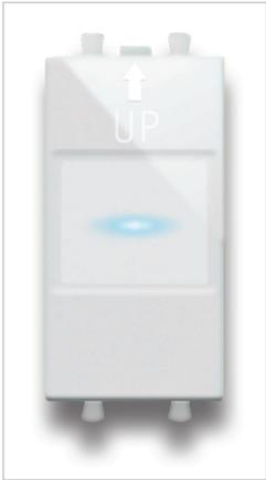
Electronic touch switch - relay output 1P NO 6A 230V~ - controlled by touching the frontal area or from multiple points with NO buttons - monostable or bistable operating mode - low consumption led for identification in the dark - output relay status memorization in case of black out - 230V~ power supply - to be coupled with Ave Touch front plate - 1 hidden module
